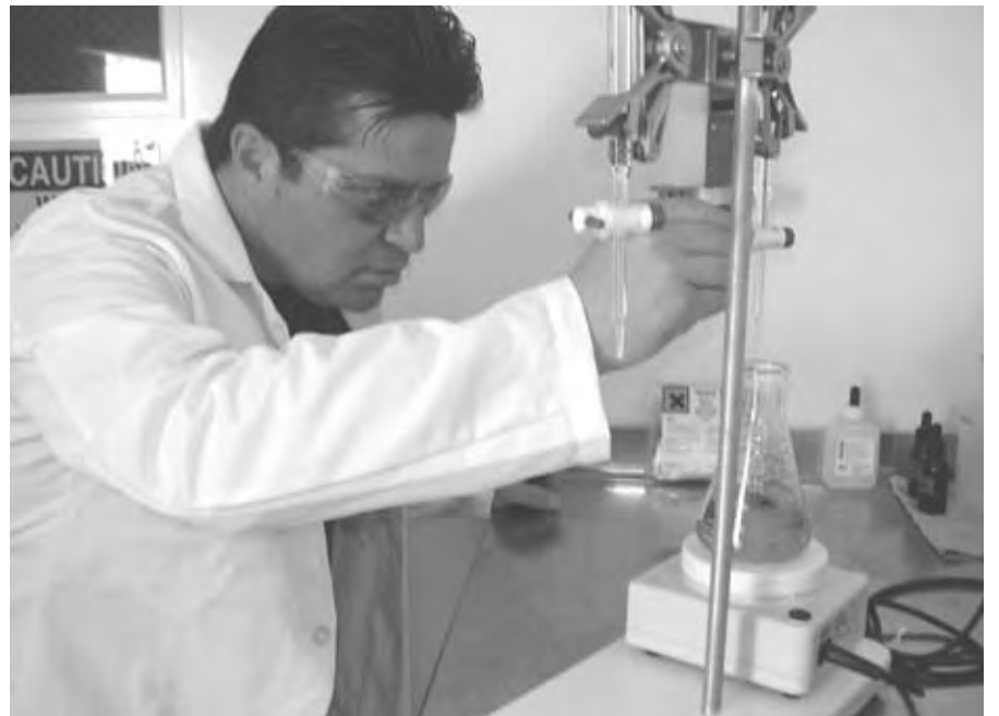
Utility Technician Gerald Romero tests pH in a water sample at the new Drinking Water Project Pilot Plant south of the Alameda Bridge in the North Valley.
